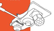
Tilt Tension Control Knob: Turn knob clockwise to tighten the tilt tension and counter clockwise to loosen tilt tension.
